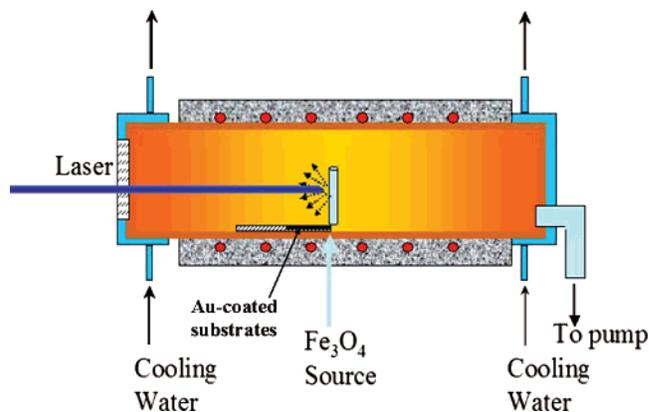
**Figure 1.** Schematic showing PLD synthesis apparatus. Laser energy is directed through a treated glass window to a pressed magnetite target. Vapors are released and re-condensed as 1D nanostructures nucleated on gold catalyst particles.
