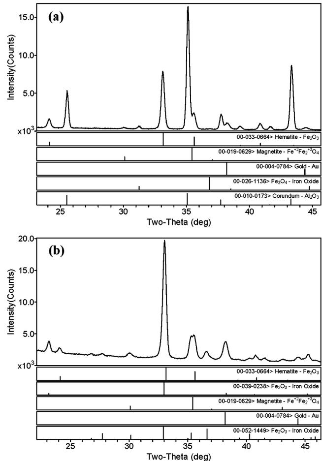
**Figure 5.** XRD data taken from samples grown at 800 °C, 10 mbar, and 750 °C 10 mbar, respectively. (a) XRD signal from grazing incidence measurements of iron oxide nanobelts and nanowires grown on polycrystalline alumina. (b) Similar measurements on iron oxide nanostructures grown on a *c*-plane sapphire substrate.
