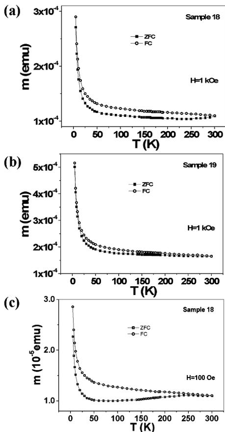
**Figure 7.** Temperature-dependent magnetization under ZFC–FC (zero field cooling–field cooling) conditions at applied field of 100–1000 Oe. (a) Effect of temperature on magnetization for iron oxide nanowire sample on alumina substrate prepared at 700 °C at 1000 Oe field strength. (b) Effect of temperature on magnetization for iron oxide nanowire sample on alumina prepared at 900 °C under 1000 Oe. (c) ZFC–FC curve for same sample as (a) under 100 Oe field strength.
